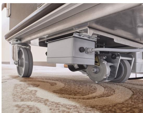
We equipped each of the 15 service trolleys with an e-drive. A control unit on the handle allows flexible control of the drive aid. If the cleaning personnel activate the e-drive, an electric drive wheel lowers and helps personnel to move the trolley. In combination with four swivel castors, specially selected to deal with this situation, the solution noticeably simplifies forward movement and makes it possible to drive the service and bar trolleys effortlessly, even on the high-pile carpet.
