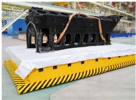
Another advantage is that all the running surfaces are polyurethane, which is good for handling characteristics and easy on the floor. Needless to say, we also approached the job within its wider context and provided AVT with a smart solution where all the components combine to form a perfect whole.
